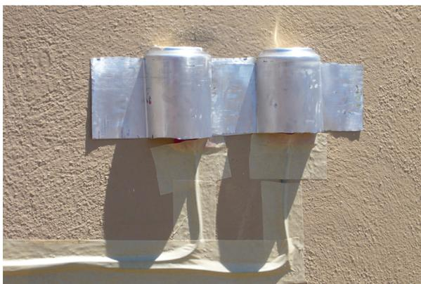
To precisely locate the surface temperature sensors at the center of the hollow and at the center solid part, an infrared camera was used to detect the surface temperature differences and locate the center of each part of the block (see Fig. 5).
