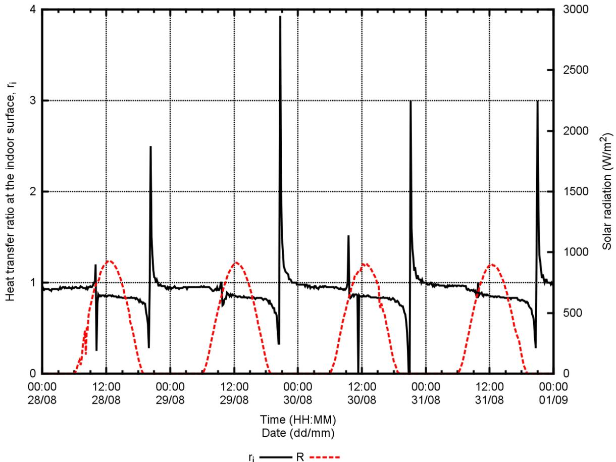
were made to study the heat transfer through the framing part (solid part) and the in-cavity path (hollow part) during four time periods from June to October 2011, (more than 30 days).
