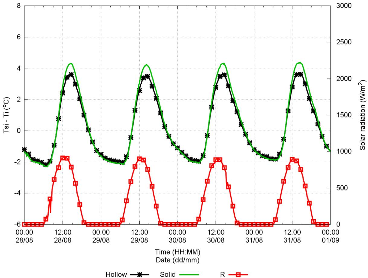
This last means that the thermal bridge is the in-cavity path for short periods. The chute-down of the curve occurs when the heat transfer at the in-cavity path changes direction, while the pique-up occurs when the heat transfer in the frame path changes direction.
