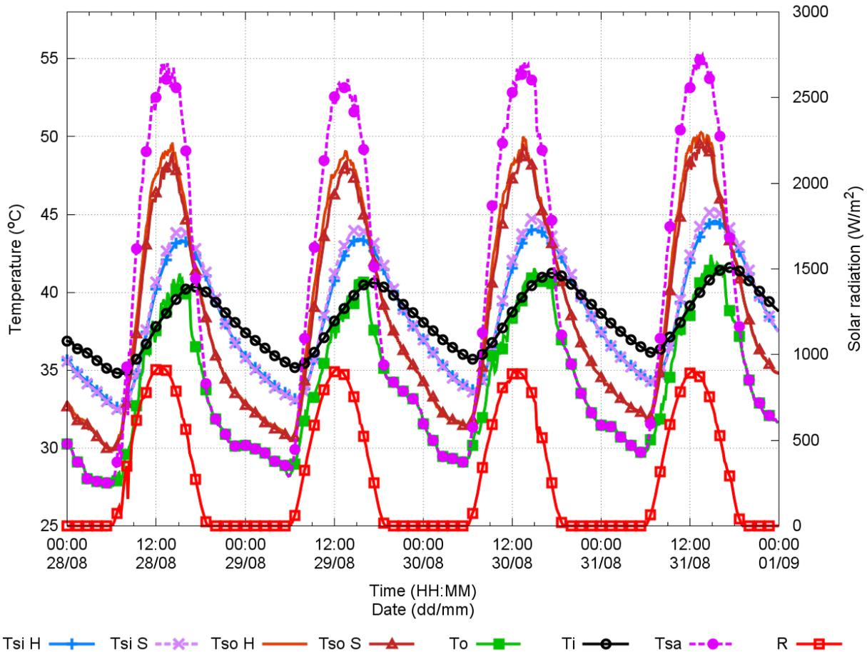
slight differences between the temperatures of both parts of the block can be appreciated.
