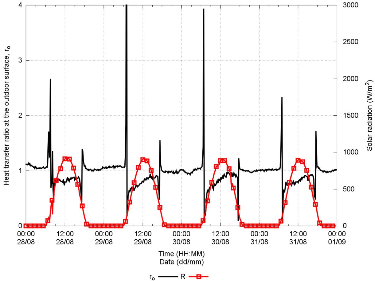
large oscillation amplitude of the outdoor air temperature, high values of the wall sol-air temperature, and high-temperature difference between wall outdoor and indoor surfaces, conditions that promote the increase of convection and radiation heat transfer through the hollow block air cavities (del Coz Díaz et al., 2011).
